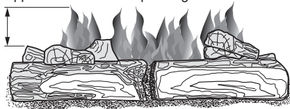
Figure 27 - Correct Burner Flame Pattern
