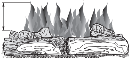
Figure 28 - Incorrect Burner Flame Pattern
