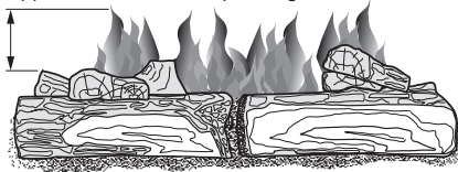
Figure 33- Correct Burner Flame Pattern
