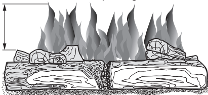
Figure 34 - Incorrect Burner Flame Pattern
