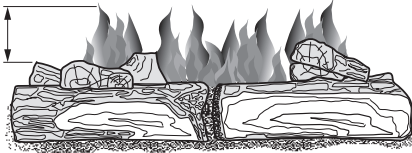
Figure 31 - Correct Burner Flame Pattern (Actual logs will vary from illustration.)
