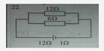
In the circuit diagram, calculate the current in the  $12\Omega$  resistor if the cell has an e.m.f of 12V and an internal resistance of  $1\Omega$ .
