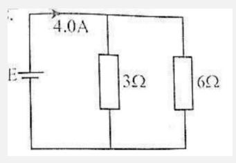
Calculate the e.m.f of the cell in the above circuit if its internal resistance is negligible.
