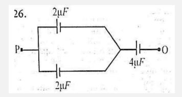
The net capacitance in the circuit shown above is \_\_\_\_\_
