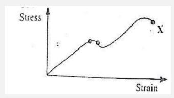
The diagram above represents the stress-strain for atypical metal rod. What does X represent?
