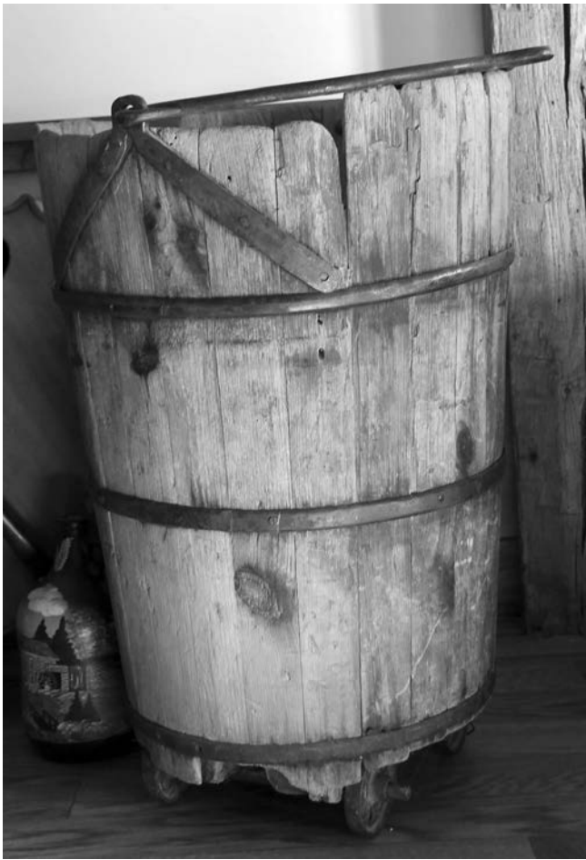
Wooden barrels were used to lift grain to the upper level of the mill until an elevator was installed in the 1900s. (Credit: Aleah Good)
