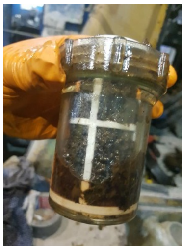
Diesel Bug & Sludge
